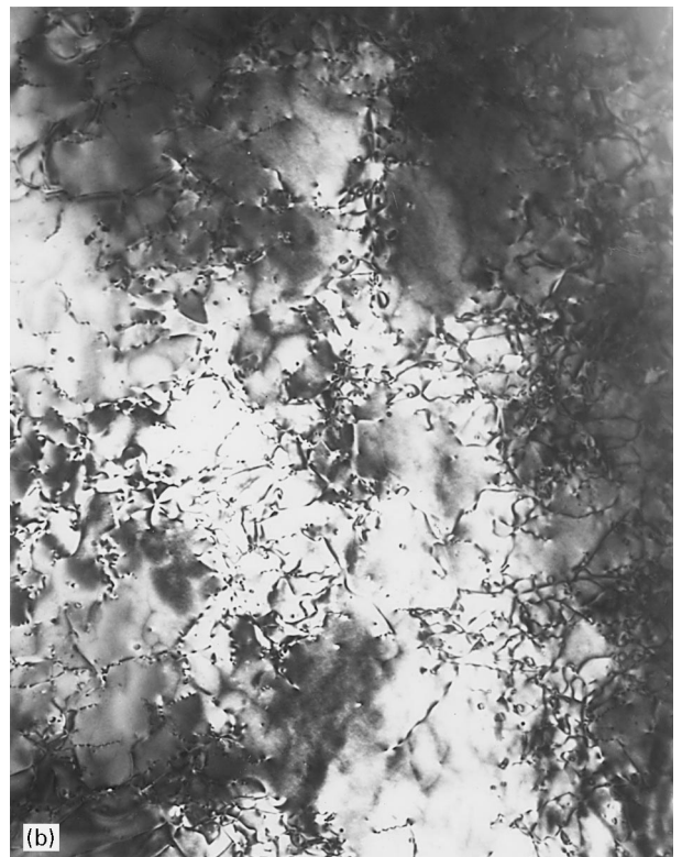
Figure 8 Transmission electron micrographs of the alloys deformed at a strain-rate of 1 \times 10^{-2} \text{ s}^{-1} to a strain level of (a) 0.5 and (b) 1.25.
